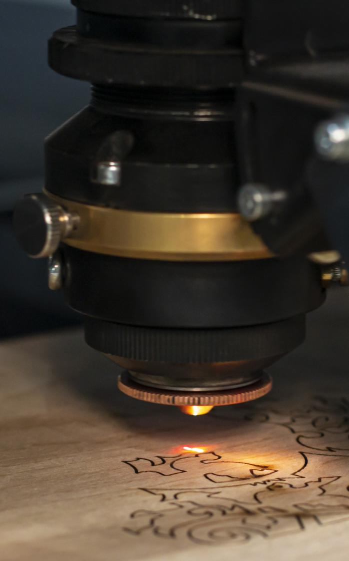
A close-up photograph of a CNC laser cutting machine's head. The metallic components are illuminated by the bright orange glow of the laser beam as it cuts through a light-colored wooden surface, creating intricate patterns.
