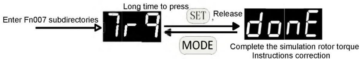
Note 1: before correcting operation, first direct short the CN2 analog voltage input port Vref (25 feet) and AGND circuit (13 feet)
