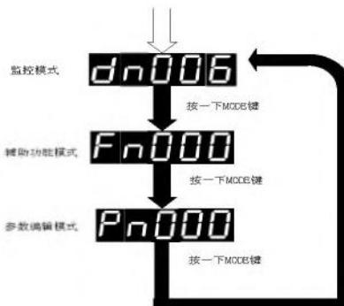
Note: when the screen shows Fnxxx, Dnxxx, Pnxxx, mode key at this time as the mode switching function, can be switched to other mode directly, otherwise the mode key is as the function of returning to the upper directory.
