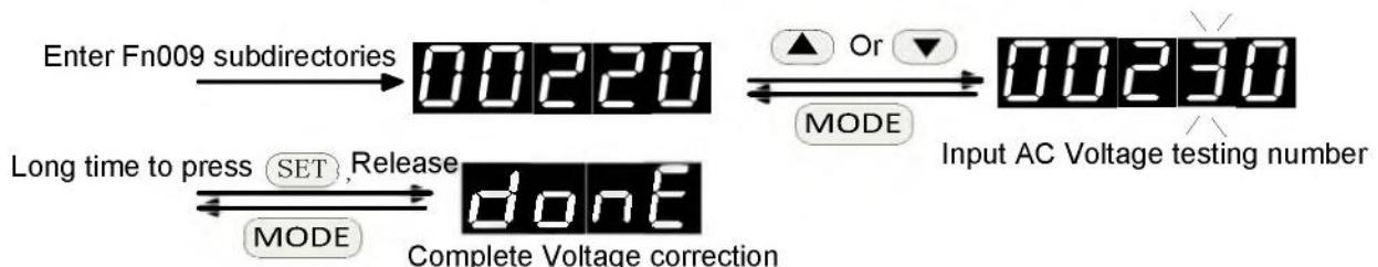
Note 1: when making correction, measurement drive input ac voltage, input to this operation.
