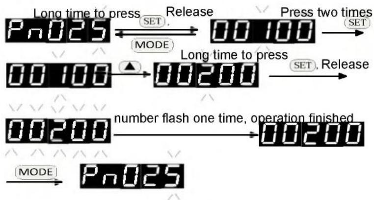
Note: Pn025 parameters are modified, if it does not have to save operation (Fn001 immortalised),
