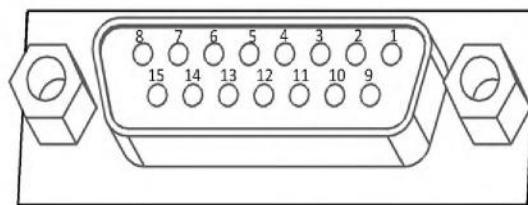
Connect the servo motor encoder signal to CN3 of the servo driver.
