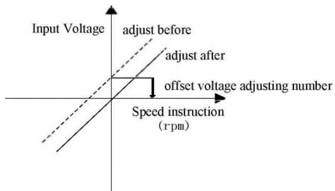
▲ Automatic offset adjusting, perform Fn008 operations.
