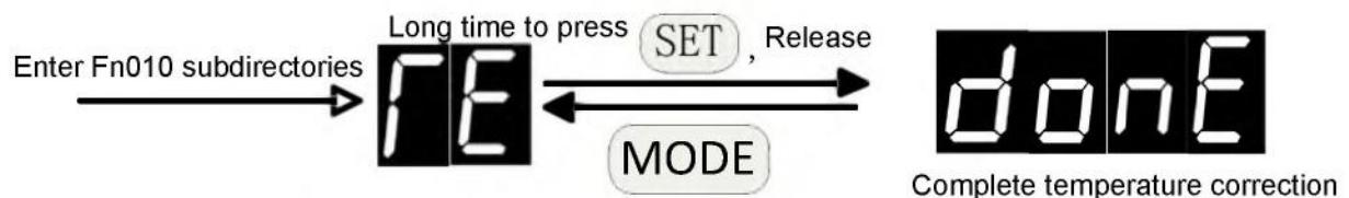
Note 1: before the operation, the temperature sensor is replaced with 1.5 K high precision resistor.
