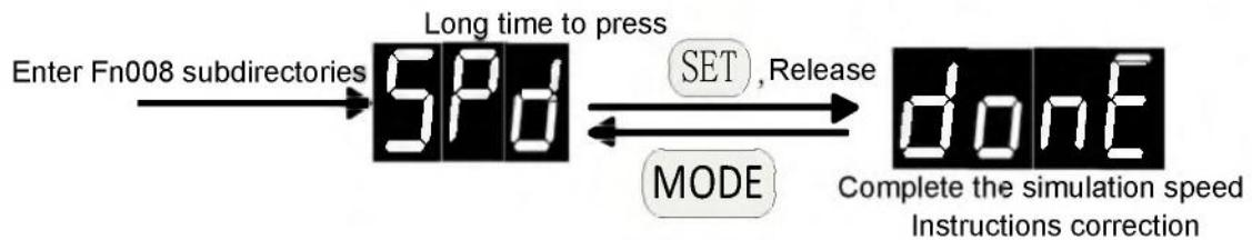
Note 1: before correcting operation, first direct short the CN2 analog voltage input port Vref (25 feet) and AGND circuit (13 feet)
