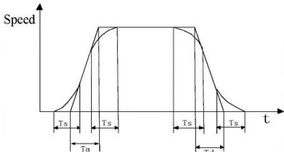
Setting Rules :  $\frac{T_a}{2} \geq T_s, \frac{T_d}{2} \geq T_s$
