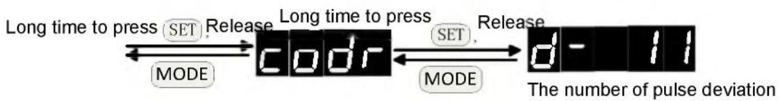
Zero before operation, confirm the motor code Pn001 set value and the actual motor model is consistent, otherwise may lead to motor current is too large, damage the motor. Adjust zero, don't need can make internal or external can make the motor, the motor will turn a few laps, and then lock the zero. When the display number of pulse bias of 0, the motor has been aimed at zero.
