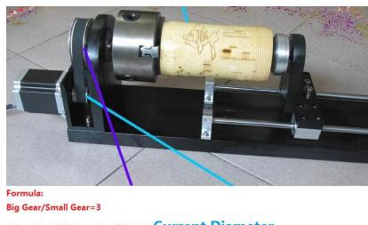
Driver Step\*(Big Gear/Small Gear)=Current Diameter
