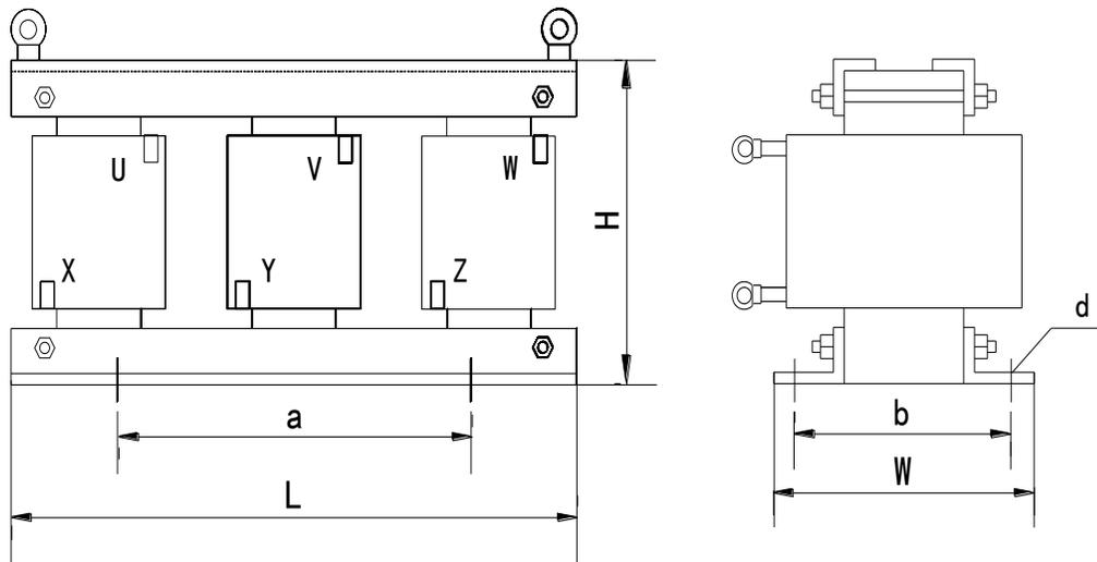
Drawing 9-2: AC input reactor dimension
