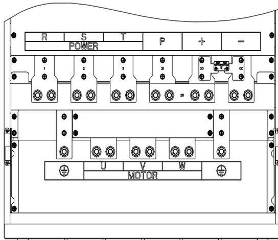
Diagram 4-11: 250kW~400kW G3 main circuit terminal
