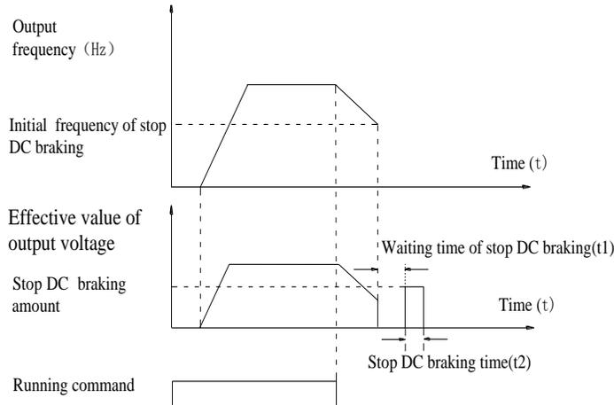
Diagram 5-9: Schematic diagram of stop DC braking time
