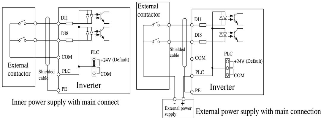
Diagram 4-14: signal input terminal circuit- dry contact mode
