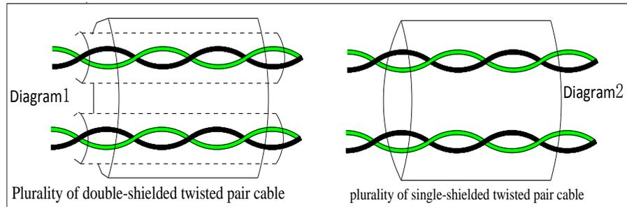
For low-voltage digital signals, double-shielded cable is the best choice, but can also be a single-shielded or unshielded twisted pair, as shown in Figure 2, however, the frequency of the signal, it can only use a shielded cable.
