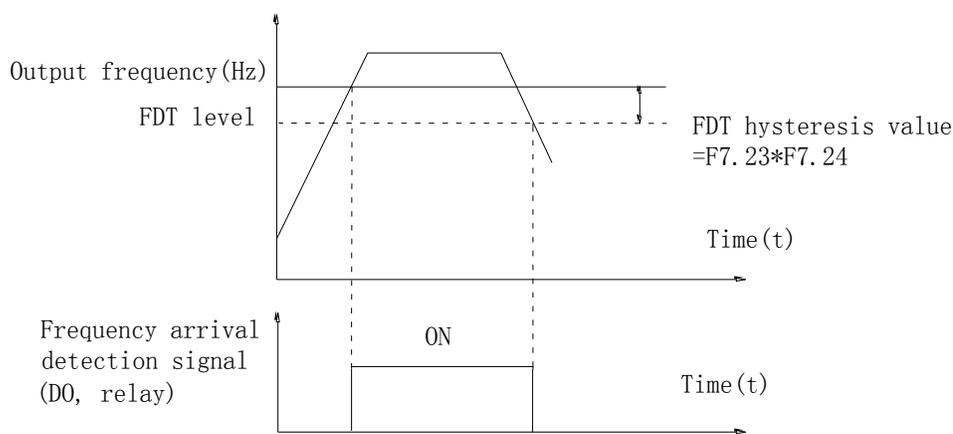
Diagram 5-22:Schematic diagram of FDT level
