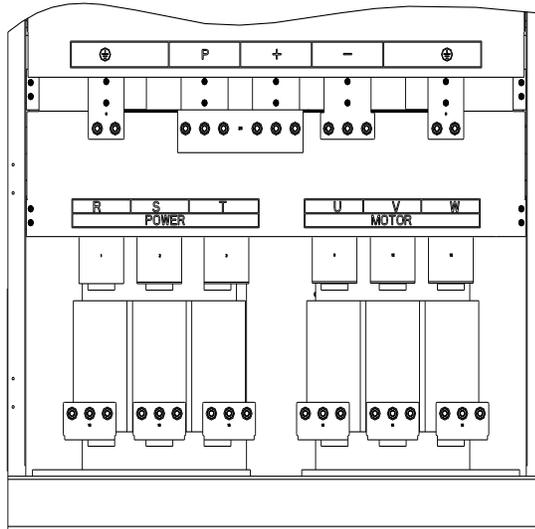
Diagram 4-12: 450kW~630kW G3 main circuit terminal
