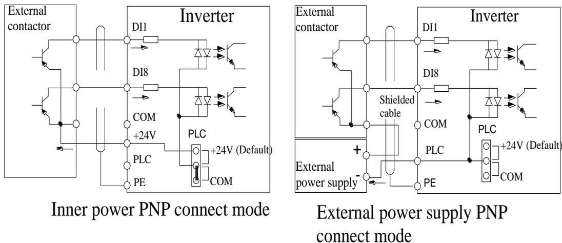
Diagram 4-16: Signal input terminal wiring diagram, open collector PNP connection mode
