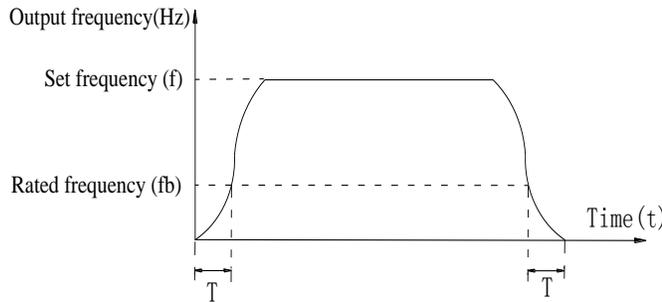
Diagram 5-11:Schematic diagram of S curve ac/deceleration B
