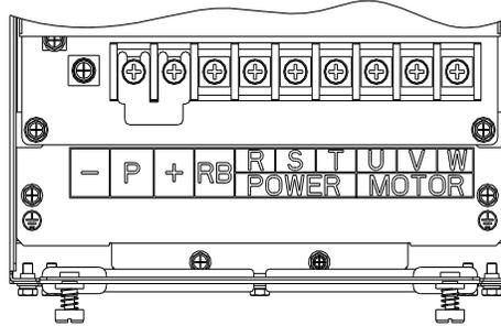
Diagram 4-5: 18.5kW~22kW G3 main circuit terminal
