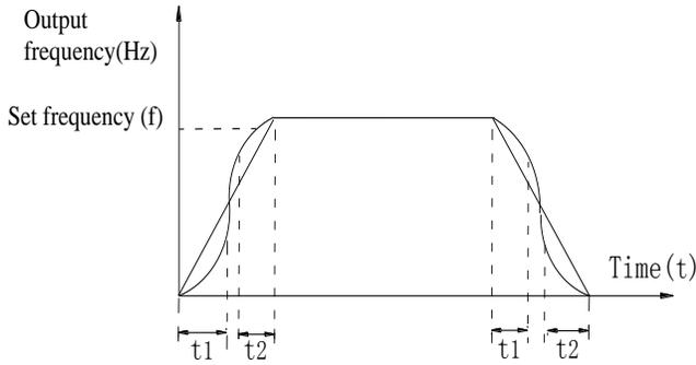
Diagram 5-10:Schematic diagram of S curve ac/deceleration A
