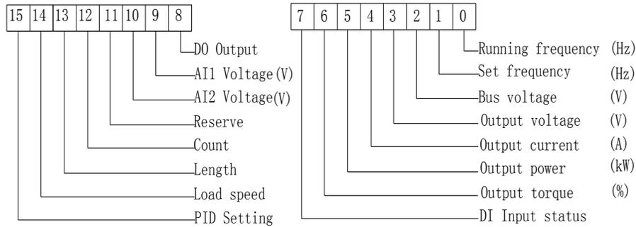
Diagram 5-15: The figure is the Running status 1
