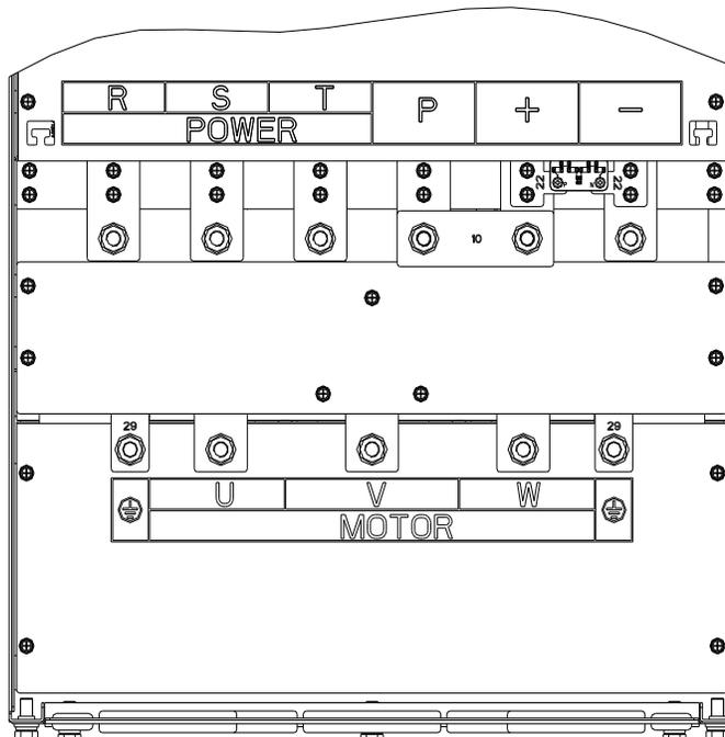
Diagram 4-10: 160kW~220kW G3 main circuit terminal
