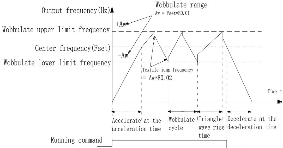
Diagram 5-29:Schematic diagram of wobble operating
