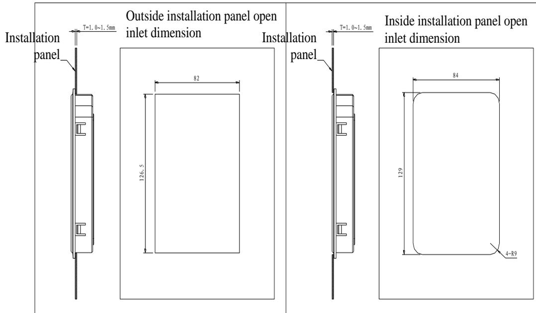
Drawing 7-7:PI500 keyboard installation open inlet dimension(mm)
