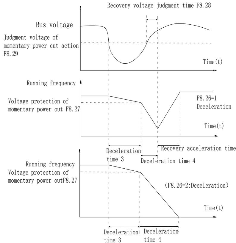
Diagram 5-28: Schematic diagram of momentary power cut action
