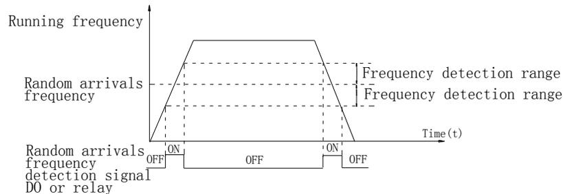
Diagram 5-24:Schematic diagram of random arrivals frequency detection
