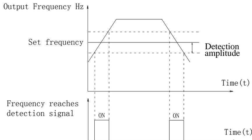
Diagram 5-23:Schematic diagram of frequency arrival detection amplitude
