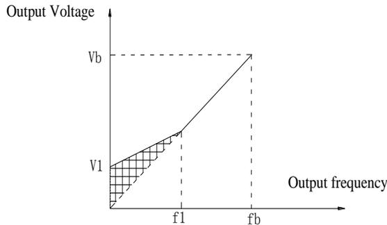
V1: Manual torque boost voltage Vb: Maximum output voltage
