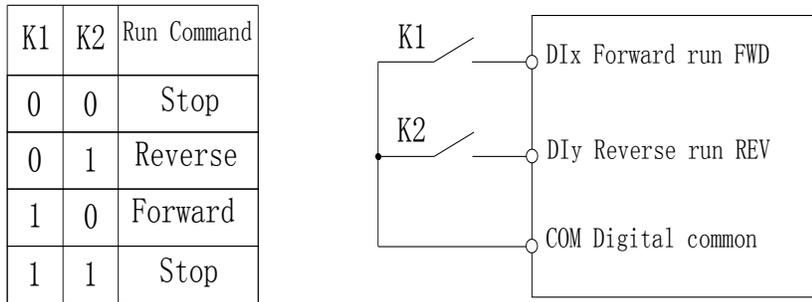
Diagram 5-3:Terminal command mode: Two wire mode 1
