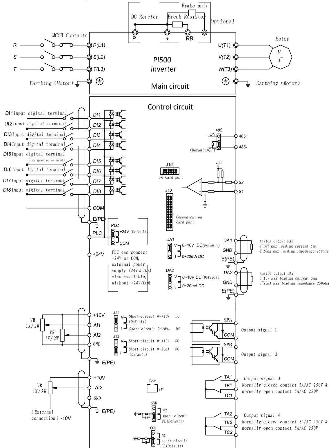
Diagram 4-3: Wiring diagram
