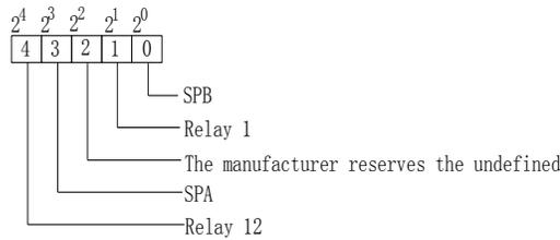
Diagram 5-2:DO the sequence of the Output terminal
