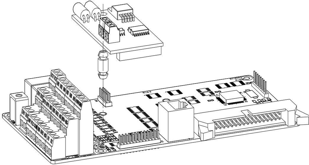
Diagram IV-1: CAN bus communication card's installation on SCB
