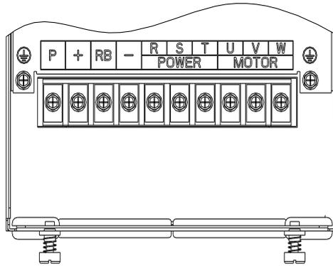
Diagram 4-4: 7.5kW~15kW G3 main circuit terminal
