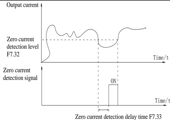
Diagram 5-25:Schematic diagram of zero current detection
