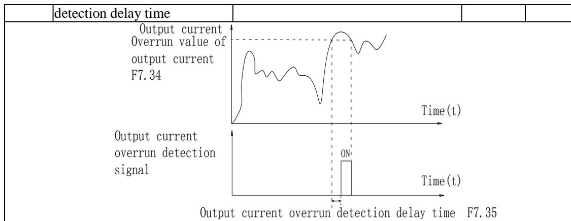
Diagram 5-26:Schematic diagram of output current overrun detection signal
