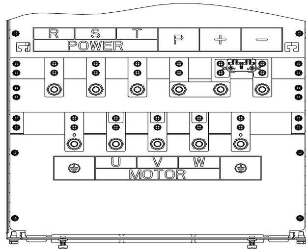
Diagram 4-9: 132kW G3 main circuit terminal
