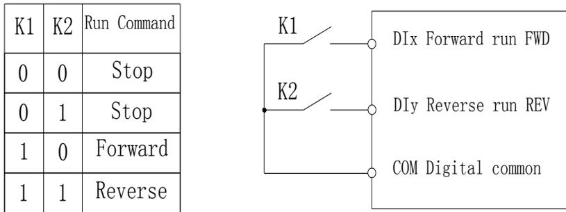
Diagram 5-4:Terminal command mode: Two wire mode 2
