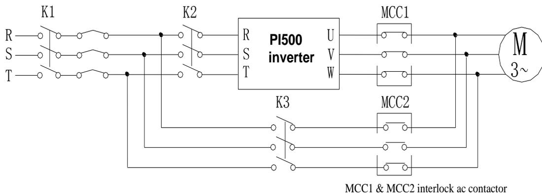
Diagram 4-17: Spare Circuit electrical diagram
