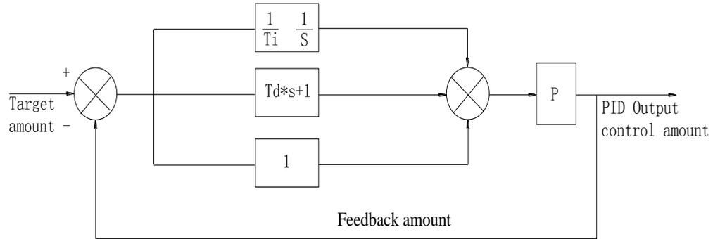
Diagram 5-32:Flow diagram of process PID principle
