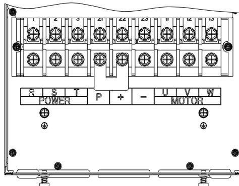
Diagram 4-7: 45kW~75kW G3 main circuit terminal
