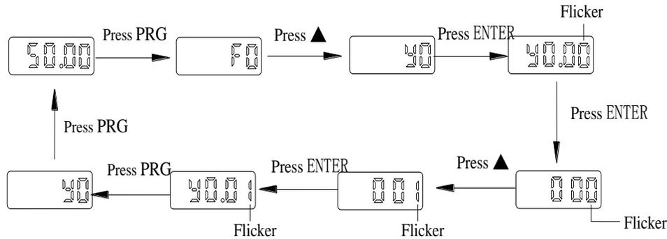
Without twinkling parameter position, the function code can not be modified in the level 3 menu. The reason maybe as following:
