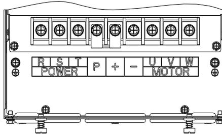
Diagram 4-6: 30kW~37kW G3 main circuit terminal
