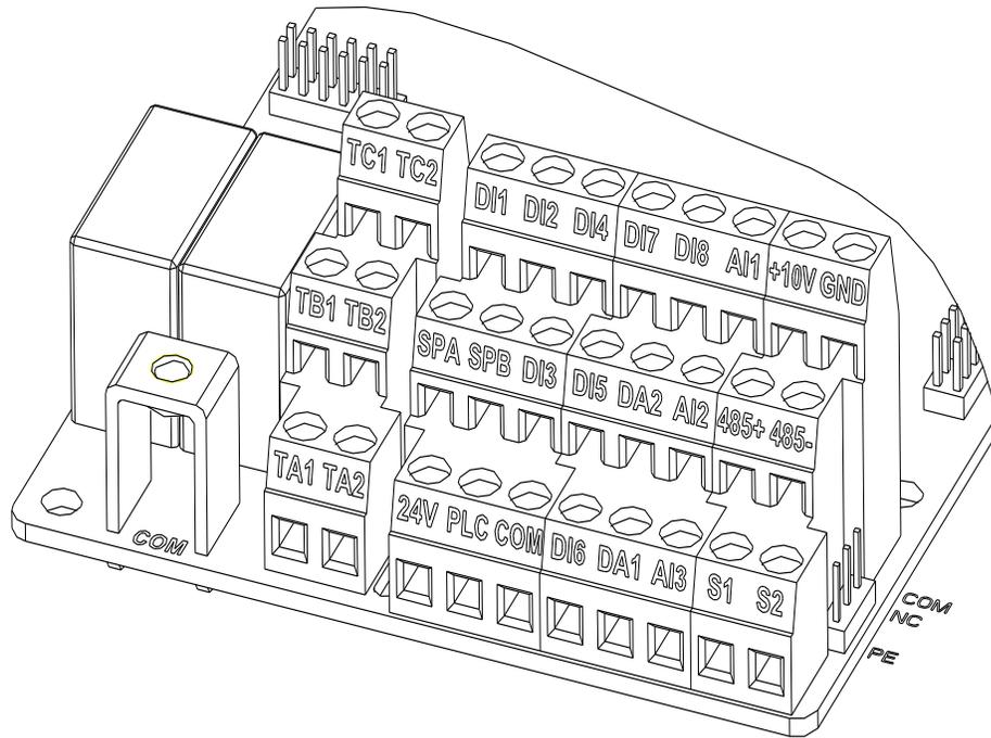
Diagram 4-13: Control panel control circuit terminals
