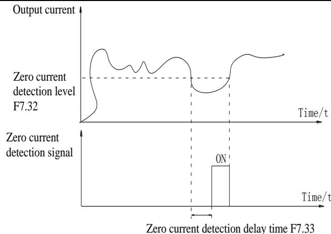
Diagram 5-25:Schematic diagram of zero current detection
