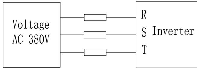
Drawing 8-1:380V Drive equipment charging circuit example
