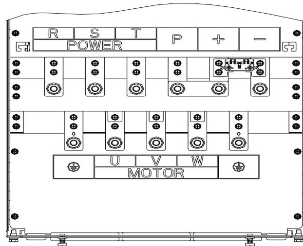
Diagram 4-9: 132kW G3 main circuit terminal
