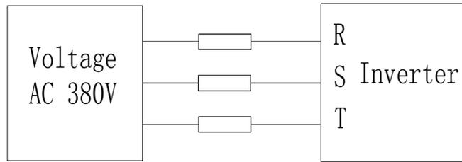
Drawing 8-1:380V Drive equipment charging circuit example
