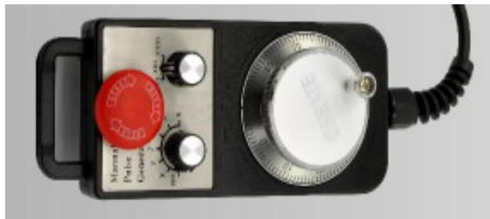
**Fig6.3 Handheld Box(Manual Pulse Generator)**
