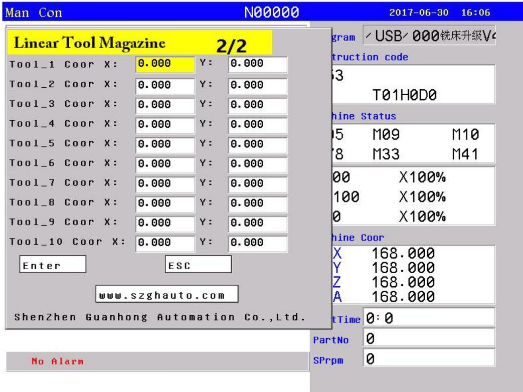
Fig5.1.3 2nd Dialog Box of Parameter Set for Linear Tool Magazine
