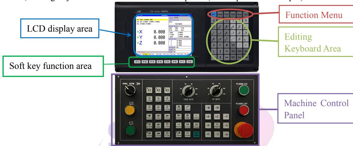
Fig.6.1 SZGH-CNC1000MDb CNC Milling Controller
