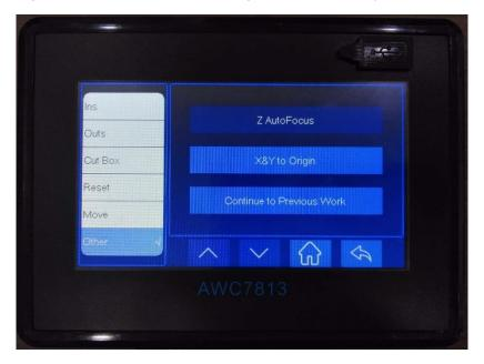
Figure 3-25 Z Autofocus, X & Y to origin and continue to previous work
