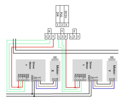
**Note:** When the Y&Z double-driver control is turned on, the Z-axis direction signal line should be connected to the Y-axis direction signal port, so that the Y&Z double-
