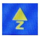
2) Z axis down move key, control Z axis to move down.
