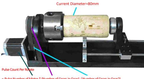
Figure 3-15-4-3 Fixture Rotate Engraving
