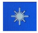
In the <u>Figure3-1-1 Main interface 1</u>, press and hold **L**aser **to** turn on laser, release this key to turn off the laser. For the content of laser power, please refer to <u>3.10.1</u> Modify Laser power.
