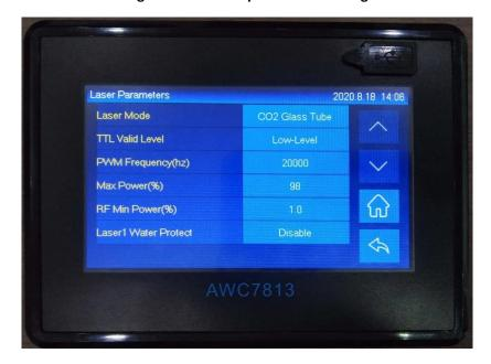
Figure 3-16-2 Laser parameters setting
