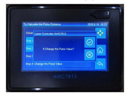
Figure 3-16-1-1-4 Modify distance per pulse
