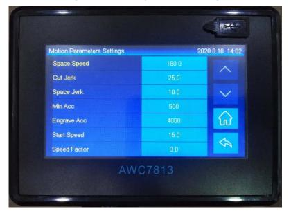
Figure 3-14 Motion parameters settings
