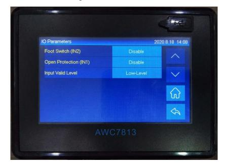
Figure 3-16-3 IO Parameters
