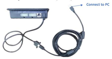
Figure 2-3-2-2 USB interface (side view)
