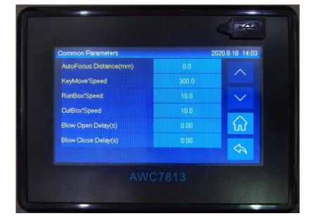
Figure 3-15-2 common Parameters
