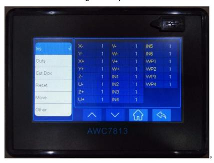
Figure 3-20 Input test
