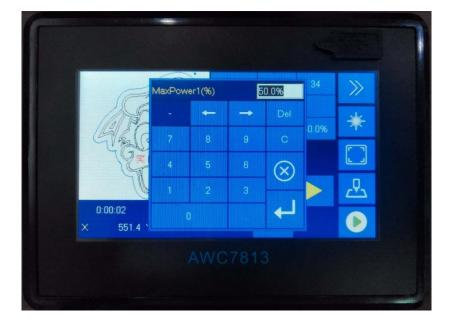
Figure 3-10-1-1 Modify the max laser power
