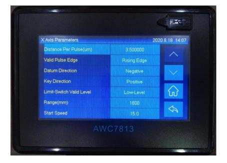
Figure 3-16-1 X axis parameters settings
