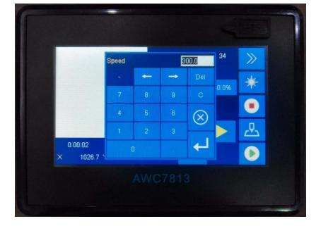
Figure 3-9-2 Modify the speed of the file being processed
