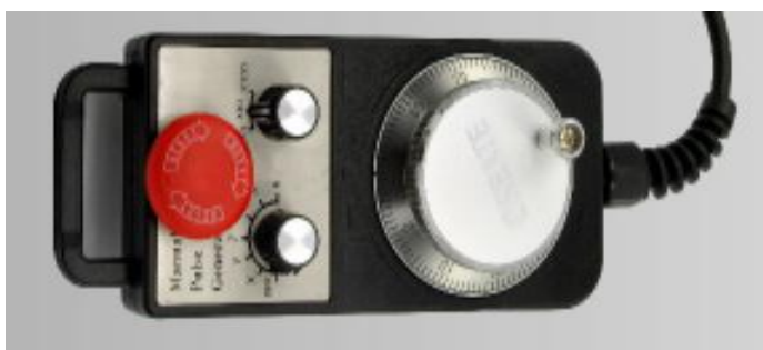
Fig1.3 Handheld Box(Manual Pulse Generator)
